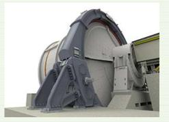
Power transmission, bearings, bushes and seals opens with an innovation from Metso Minerals about its newly released mill drive system. The QdX4 Mill Drive system is an advance on dual-pinion drives into a quad pinion system. Two electric motors with torque splitting systems are used to drive two pinions each. The system enables high transmission efficiencies for large ball and SAG mills operating at between 18 kW and 28 kW.
