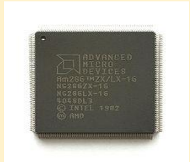
Fig: a. Exynos 4 Quad (4412) System on a Chip AMD b. Am286ZX/LX, SoC based on Intel 80286
