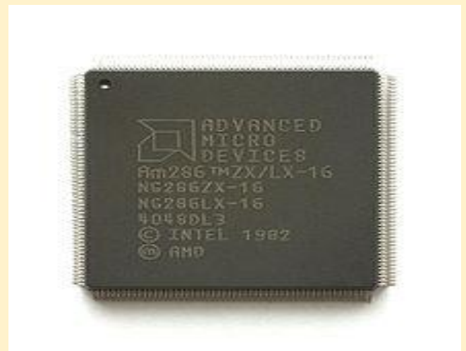
Fig: a. Exynos 4 Quad (4412) System on a ChipAMD b. Am286ZX/LX, SoC based on Intel 80286
