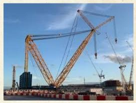
The SGC-250 stands an astonishing 820 feet at its tallest point, has a maximum lift capacity of 5500 US tons and a swing radius of over 900 feet. The behemoth will be a key component in the construction of the Hinkley Point C nuclear power station in South West England.
